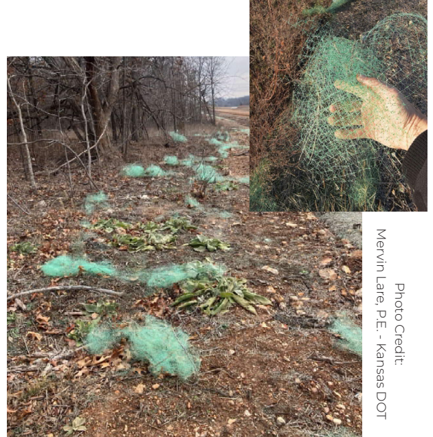
Photodegraded netting clumping up & blowing off the project like a tumble weed. This is now trash that needs cleaned up.
