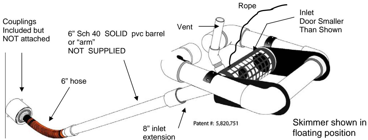
2. Glue the 6" sch 40 barrel at least 8' long to the 6" dark coupling on the hose.
